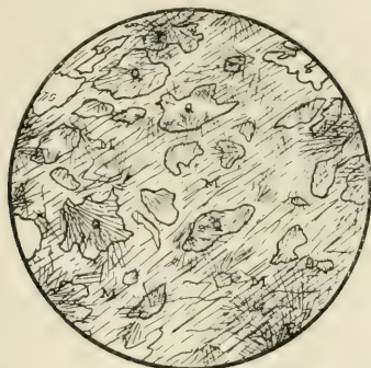
Appearance of nodules in thin section. M Silvery Mica, Q Quartz, F Fibrolite. X 14.
